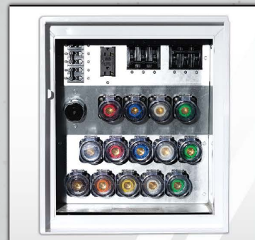
5 | Simultaneous Voltage Output Panel 120V - 20A x 2 | 240V - 50A x 1 3Φ 240V & 3Φ 208/480v Cam-Loks™
