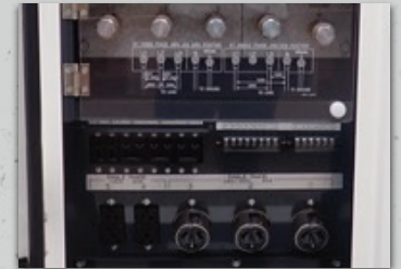
2 | Output Panel 120V - 20A x 2 | 240V - 50A x 3 with Terminal Block for VFD Remote Control
