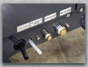
11 | Exterior Service Drains Quick drain valves for Fuel, Oil Cooler, Radiator and Engine Oil fluids
