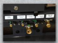
8 | Exterior Service Drains Quick drain valves for Fuel, Oil Cooler, Radiator and Engine Oil fluids
