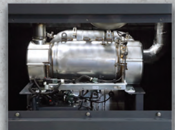
13 | Front-mounted SCR System Convenient access for easy servicing
