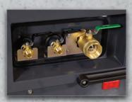
**3** | Air Connections 3/4" Ball Valve x 2 | 2" Ball Valve x 1
