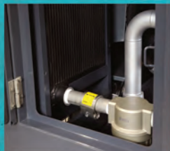
Integrated After Cooler
