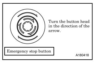
After emergency stopping, be sure to carry out an investigation of the cause you made stop and the countermeasure, release emergency stop button after making sure the safety was confirmed.
