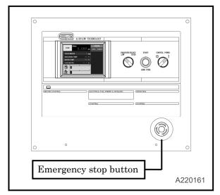
• If it is necessary to stop the machine for emergency, press the Emergency Stop button which set up under part of the operation panel.
