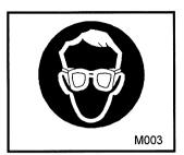
When cleaning dust accumulated in such devices as the air-filter, by blowing compressed air, wear safety glasses, etc. to protect your eyes.
