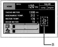
• The exhaust temperature may not reach temperatures hot enough to burn soot during operation in cold weather or under low loads. If the unit is operated under low load or in cold weather for an extended time, a DPF indicator [B] will be displayed. Immediately take action and being a Manual Regeneration by following steps below.
