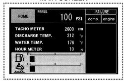
When an alert or fault occurs, an indicator will blink.
