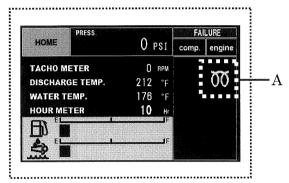
4. Once the glow lamp [A] is extinguished, press the [START] button for 1 second or longer to start the engine.
