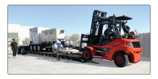
**2)** Position the pintle hitch attachment to connect to the EBOSS<sup>™</sup> trailer. Slowly raise the forks to level out the EBOSS<sup>™</sup>. Carefully begin backing the EBOSS<sup>™</sup> off of the flatbed trailer.
