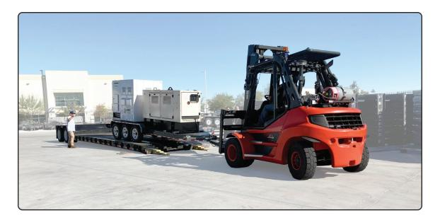
**4)** Carefully lower the forks, positioning the EBOSS<sup>™</sup> onto the flatbed trailer. Disconnect the pintle hitch and slowly back the forklift away from the trailer. Attach rigging required to secure the load.
