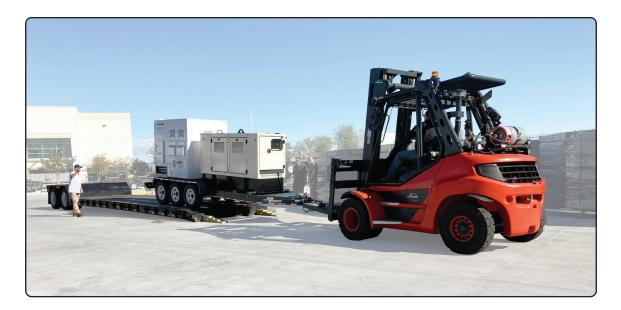
**4)** Back the EBOSS<sup>™</sup> completely away from the flatbed trailer. Engage the trailer jacks into an upright position and lower the forks to set the EBOSS<sup>™</sup> on the ground. Disconnect the pintle hitch.
