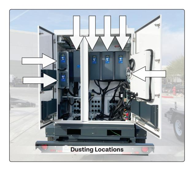
Compressed air should be used to remove dust and debris from the EBOSS™. Do not make contact between the air nozzle and the sensitive electronics of the EBOSS™, as damage can result.
