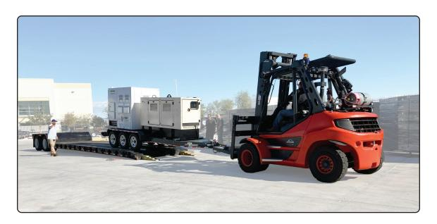
**4)** Back the EBOSS<sup>™</sup> completely away from the flatbed trailer. Engage the trailer jacks into an upright position and lower the forks to set the EBOSS<sup>™</sup> on the ground. Disconnect the pintle hitch.
