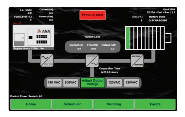
The top left of the screen above the generator shows, line voltage (VAC), current (A), fuel level (%) and power (kW) output of the generator. When the start button is pressed the generator status will display the following:
