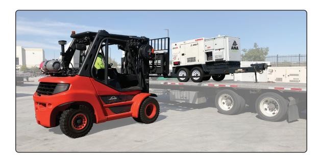
**2)** Position forks to lift behind the rear axle and forward of the front axle to balance the load. Slowly raise the forks until making contact with the EBOSS $^{\text{\tiny{M}}}$ . Carefully lift the EBOSS $^{\text{\tiny{M}}}$  up off the trailer.
