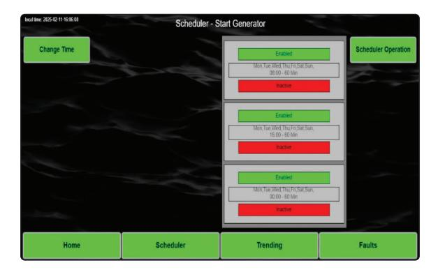
Please note the local time in the upper left corner and ensure its accuracy before enabling the scheduler. Adjust if necessary.
