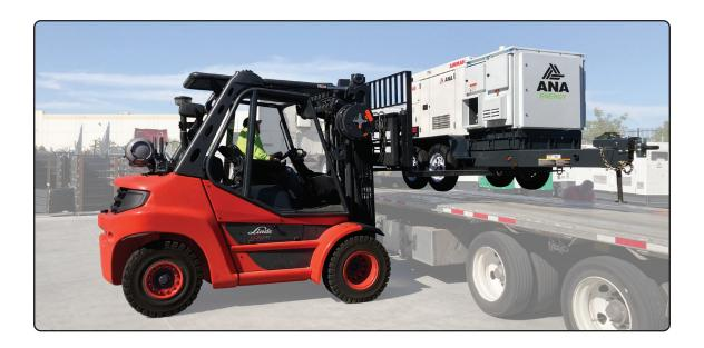
**4)** Carefully lower the EBOSS<sup>™</sup> onto the flatbed trailer. Lower the forks slowly to ensure the load is stable on the trailer. Once forks are clear of the EBOSS<sup>™</sup>, slowly back forklift away from the trailer.
