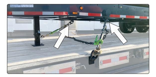
Tie down locations are located in front of the front axles (2) and behind the rear axles (2). These are designed for tie down only and are not designed for lifting the EBOSS<sup>™</sup>.
