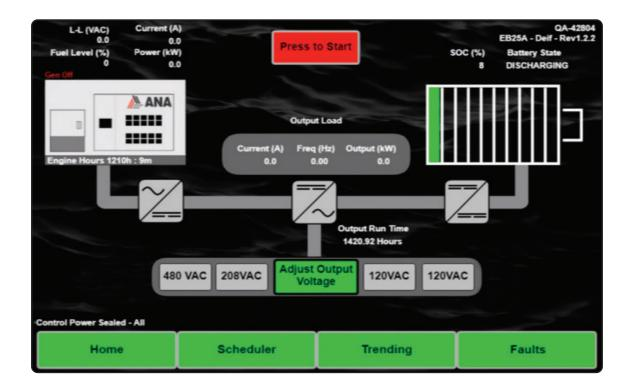
The top left of the screen above the generator shows, line voltage (VAC), current (A), fuel level (%) and power (kW) output of the generator. When the start button is pressed the generator status will display the following:
