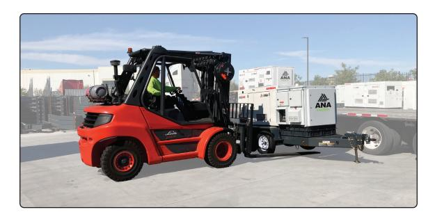
**2)** Slowly raise the forks until making contact with the EBOSS<sup>™</sup>. Carefully lift the EBOSS<sup>™</sup> up off of the ground. Ensure the EBOSS<sup>™</sup> is balanced on the forks.
