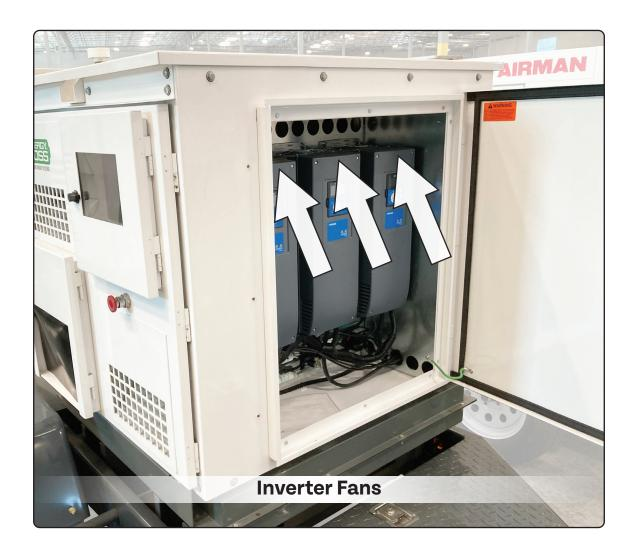
Compressed air should be used to remove dust and debris from the fans. Do not make contact between the can nozzles and the sensitive internal electronics of the EBOSS $^{\text{\tiny M}}$ , as damage can result.
