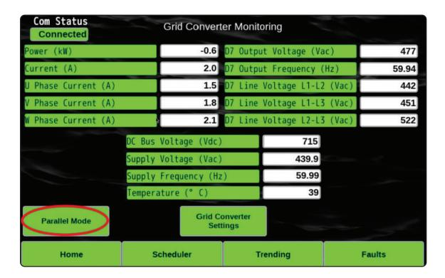
Once all units to be paralleled have the parallel selection set, start one of the units and enable the output, then bring all other units online (there is no number or timing sequence).
