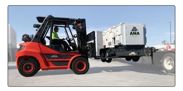
**4)** Slowly lower the forks, placing the EBOSS<sup>™</sup> on the ground. Lower the forks a few more inches, so they fully clear the EBOSS<sup>™</sup>. Carefully back the forklift away from the EBOSS<sup>™</sup>.
