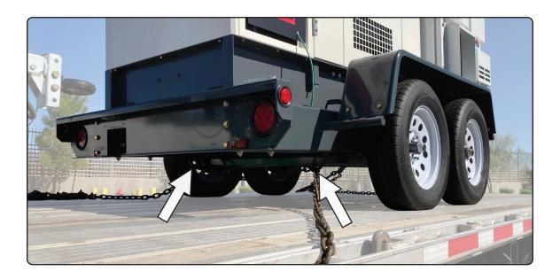
Tie down locations are located in front of the front axles (2) and behind the rear axles (2). These are designed for tie down only and are not designed for lifting the EBOSS $^{\text{\tiny M}}$ .
