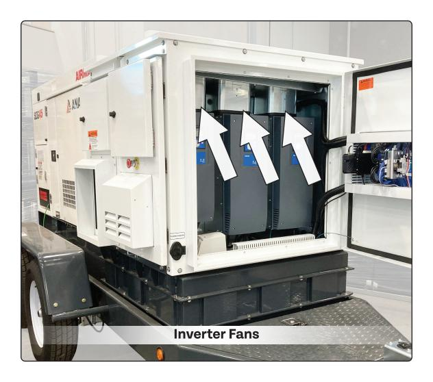
Compressed air should be used to remove dust and debris from the fans. Do not make contact between the can nozzles and the sensitive internal electronics of the EBOSS $^{\text{\tiny M}}$ , as damage can result.
