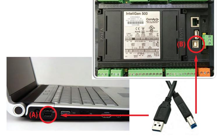
Locate the USB ports (A) and (B) on the laptop and the back of the ComAp controller.
