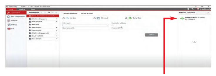
If the connection is proper, the program will auto detect the ComAp controller.
